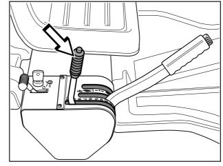
**4.** Push in the lock button on the lift lever and lower down the cutting unit.
